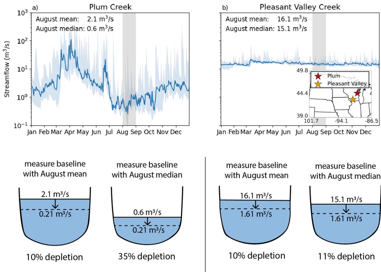
**Fig. 5.** Plum Creek has a highly variable annual hydrograph (a), whereas Pleasant Valley Creek is very stable (b). In this example, we assume that groundwater pumping at both sites results in a 10% reduction of streamflow from the mean August streamflow. This same streamflow reduction could be measured as a 35% depletion from the August median for Plum Creek or 11% for Pleasant Valley Creek.
