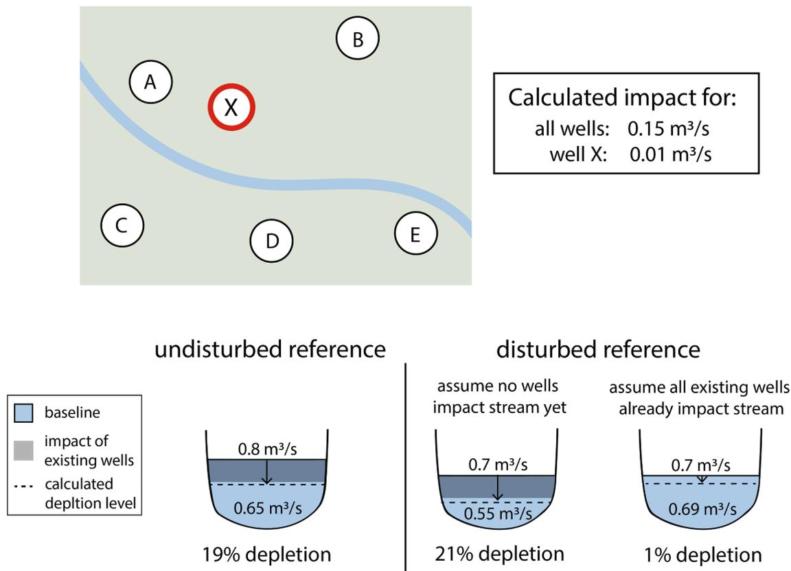
**Fig. 4.** Choices and assumptions that define a hydrological reference condition have a large impact on streamflow depletion calculations. This demonstrative example shows more than an order of magnitude difference in depletion calculations given different reference conditions: an undisturbed reference and a disturbed reference for which two different assumptions are made about current impacts on the stream.
