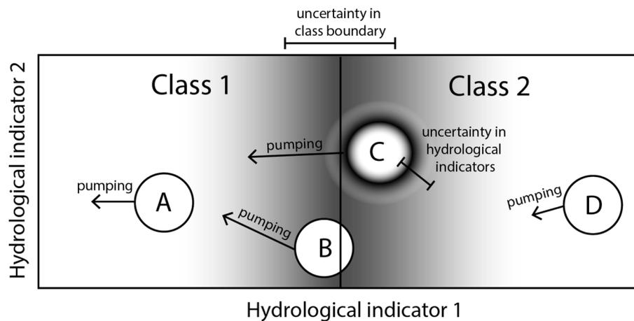
**Fig. 6.** Uncertainty in class boundaries and stream quantities can impact stream classification. Stream A is clearly in Class 1. Stream B appears to be in Class 1 but could be in Class 2 if the class boundary moves within the uncertainty bound. Stream C appears to be in Class 2, but uncertainty in the stream quantity means that it could be in Class 1. Arrows show potential trajectories for streams given changes that could occur with streamflow depletion.
