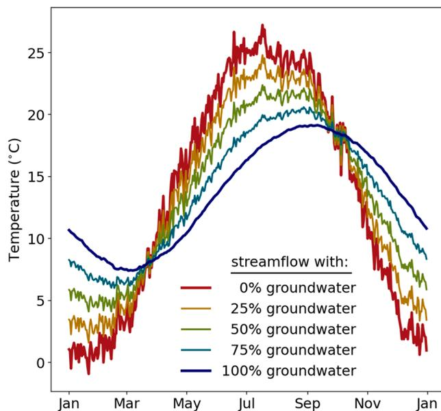
Fig. 7. Schematic demonstrating the difference in thermograph for streamflow that consists of 100% groundwater (navy) and 0% groundwater (red). As the groundwater contribution to streamflow increases, as shown with the examples for 25%, 50%, and 75% groundwater, the streamflow thermograph shifts closer to the 100% groundwater thermograph.
